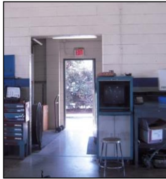
Figure 7: A potential path of migration created by an open passageway. Photo courtesy of Gladstein, Neandross & Associates, NREL
